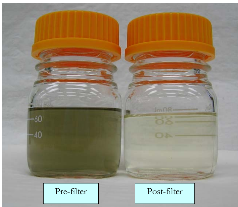
Photo 5-2: Comparisons of Pre- and Post-filtered Syn-gas Acetone-tar Solutions
